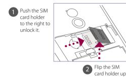
nsert the USIM/SIM card with its gold 3 ontacts facing down and its cut-off corner facing the battery compartment.
